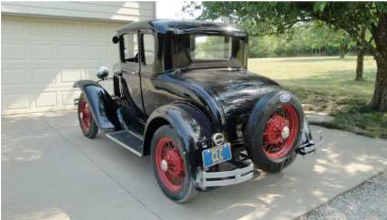
Between March and June of 2012, the body work was completed and the car was painted, assembled, new glass installed, wired with new lighting installed, new seat, door panels and kick panels installed. The car still needs a headliner installed and the bumpers rechromed, but it was complete enough to be returned to Floyd.
